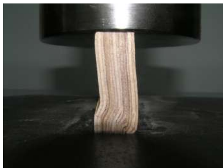
Figure 1: Test specimen during testing the compressive strength of experimental plywood
