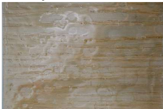
Figure 2: Problem in the wetting of the water-based base coating by the following epoxy coating (Palija, 2020)
