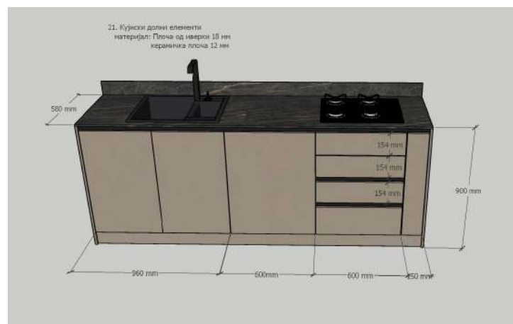
Figure 7: 3D model of kitchen base cabinets (position no.21 in the element database)
