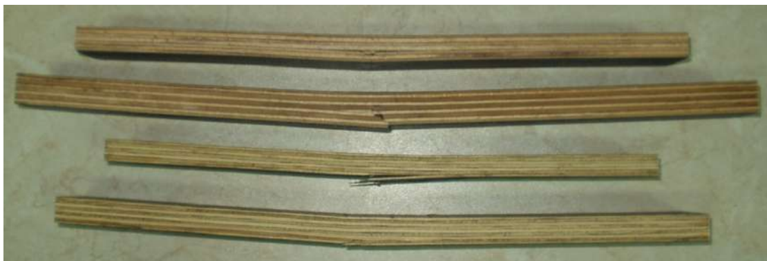
Figure 2: Failure mode of the test specimens of the experimental panels
