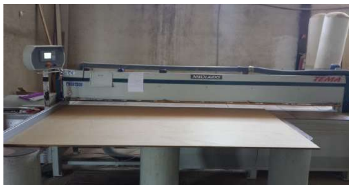
Figure 1: Circular saw machine type NIKOLAIDIS TEMA 3800
