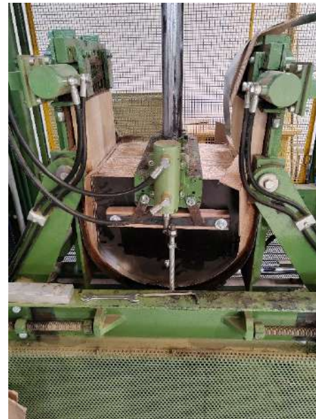
Figure 2: Mechanical press during bending
