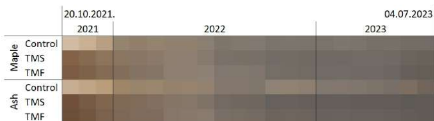
Figure 4: Heatmap visualization of color change during the weathering test
