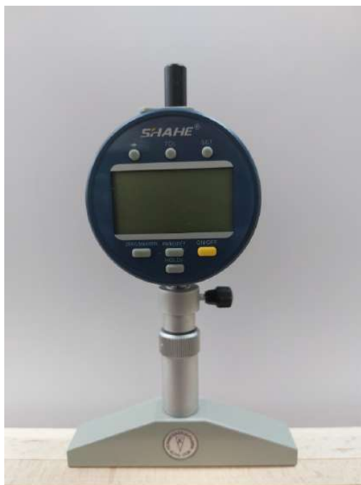
Figure 3: Digital comparator for measuring roughness type Shane
