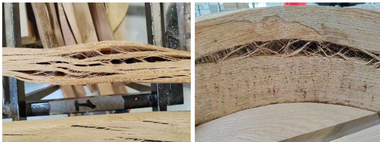
Figure 3 and 4: Cracks and gapes in wood tissue due to excessive HF heating
