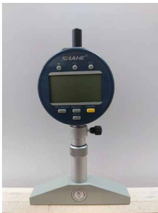
Figure 3: Digital comparator for measuring roughness type Shane
