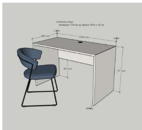
Figure 2: 3D model of a work desk (position no. 8 in the element database)
