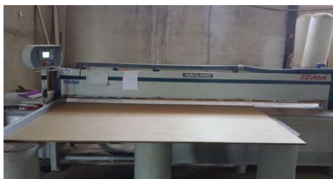
Figure 1: Circular saw machine type NIKOLAIDIS TEMA 3800
