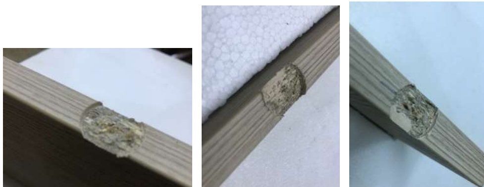
Figure 4: Characteristic damage of the samples after the test (from left to right, samples of group 1 to group 3)
