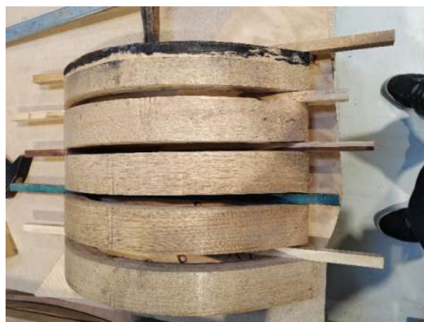
Figure 7: Chair backs after bending
