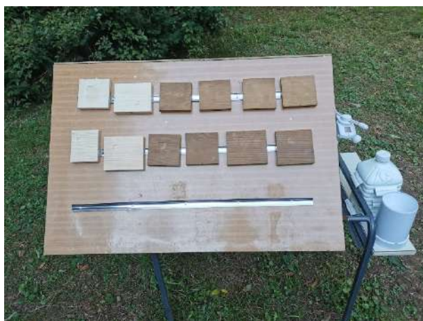
Figure 1: The setup for weathering test
