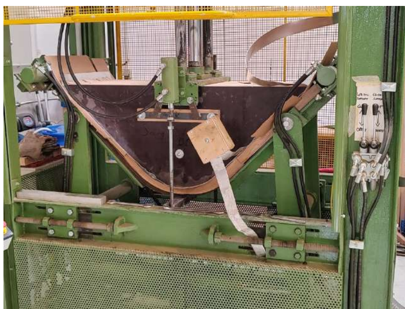
Figure 5: Heating specimens, capacitor can be seen added to the press
