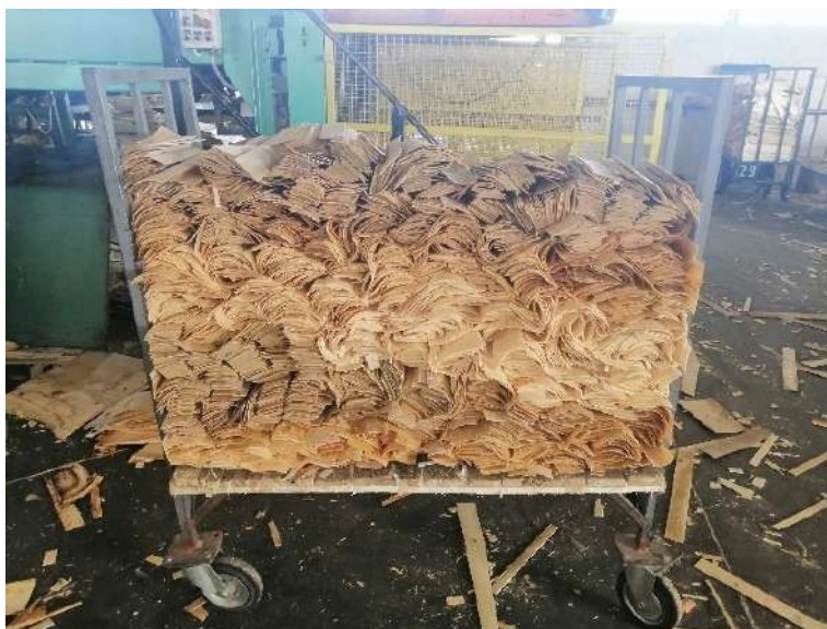
Figure2: Elements after peeling of poplar logs
