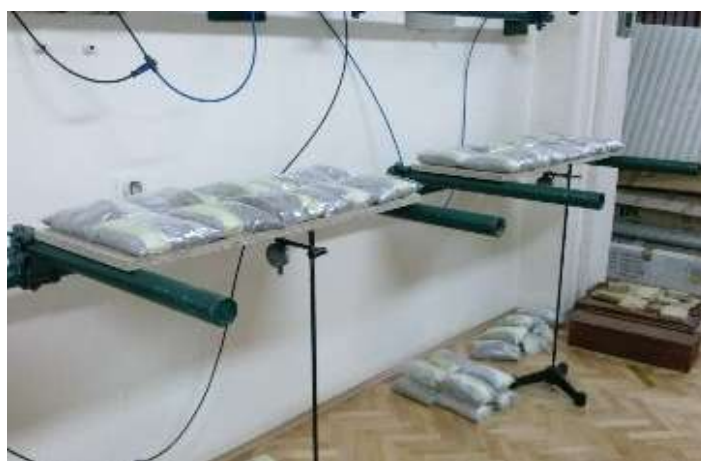
Figure 1: The testing method for bending creep behavior
