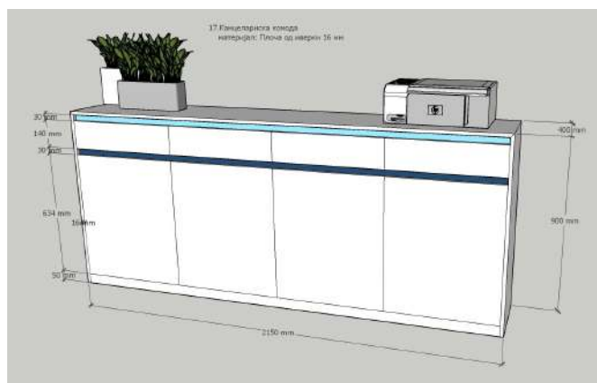
Figure 4: 3D model of a office storage cabinet (position no.17 in the element database)
