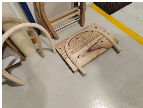
Figure 13: Turned chair pieces bent in two planes
